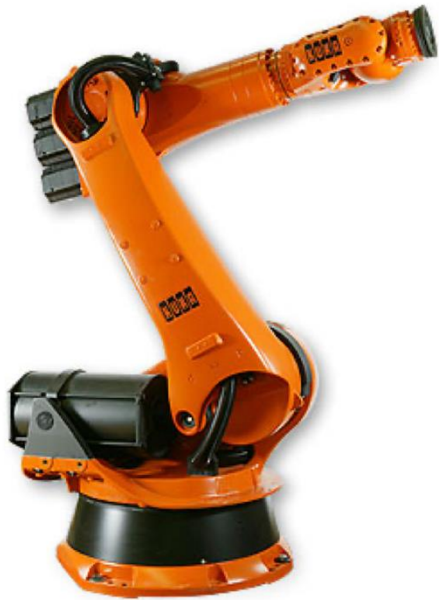
Kuka 150_2 S2000 open kinematic chain (series of rigid bodies connected by joints)
