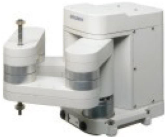
Mitsubishi RP (repeatability 5 micron, payload 5 kg)
