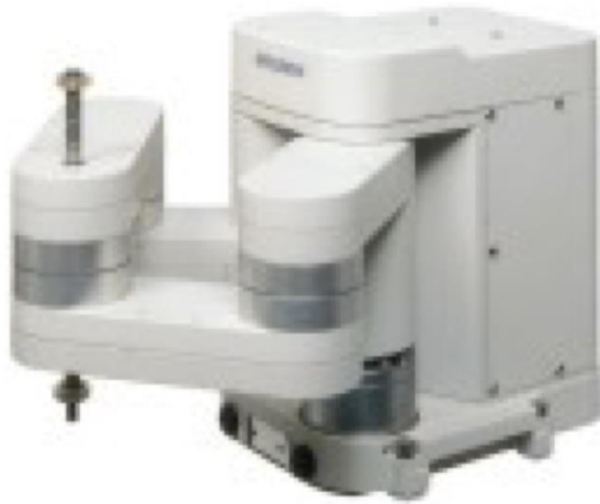
Mitsubishi RP (repeatability 5 micron, payload 5 kg)
