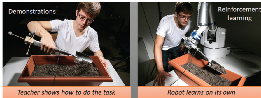
Figure 6.1: Data for training robots can either be provided by human demonstrations or gathered by the robot on its own through trial and error (known as reinforcement learning, or RL). The two modes can be combined. Demonstrations can be used to bootstrap the search, providing a good example of how to move the tool. Trial and error can then be conducted in a restricted search space around the demonstrated trajectory to gather more information on the force and impedance to apply when interacting with gravel.
