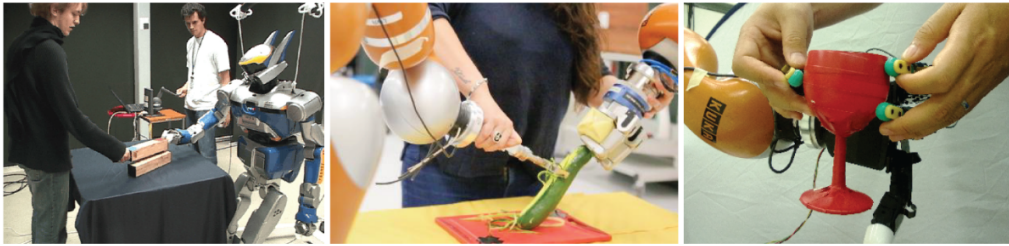
Figure 6.4: Left figure: Demonstration of a task requiring force control through teleoperation via a haptic interface. Middle figure: Example of kinesthetic teaching, in which the human puts herself in the robot's shoes to teach the robot how to peel vegetables. Forces are measured through tactile sensors at the robot's end points. Right figure: Example of kinesthetic teaching to teach how to manipulate an object. Forces are measured through tactile sensors at the robot's fingertips.
