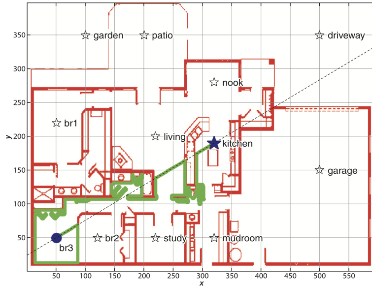
Figure 3.3: Obstacles are indicated by red pixels . Named places are indicated by hollow black stars . Approximate scale is 4.5 cm per cell. The start location is a solid blue circle and the goal is a solid blue star . The path taken by the bug2 algorithm is marked by a green line . The black dashed line is the m-line, the direct path from the start to the goal
