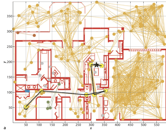
Figure 3.11: Probabilistic roadmap (PRM) planner showing the path taken by the robot via nodes of the roadmap which are highlighted in yellow
